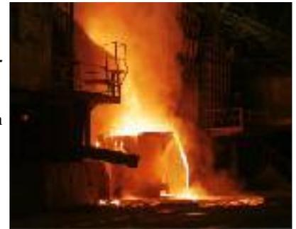
The FeO and MnO are generally the most destructive compounds in the bath. Reducing the FeO and MnO with *POWERMELT* can often double lining life. Keep in mind, the level of improvement depends on the amount of iron oxide that is introduced to the furnace. While rusty scrap or too much preheating will add to the FeO problem, clean charge materials will enhance lining life. Then again, as scrap quality varies SiC acts as a safeguard removing more
