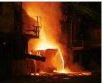
The FeO and MnO are generally the most destructive compounds in the bath. Reducing the FeO and MnO with POWERMELT can often double lining life. Keep in mind, the level of improvement depends on the amount of iron oxide that is introduced to the furnace. While rusty scrap or too much preheating will add to the FeO problem, clean charge materials will enhance lining life. Then again, as scrap quality varies SiC acts as a safeguard removing more
